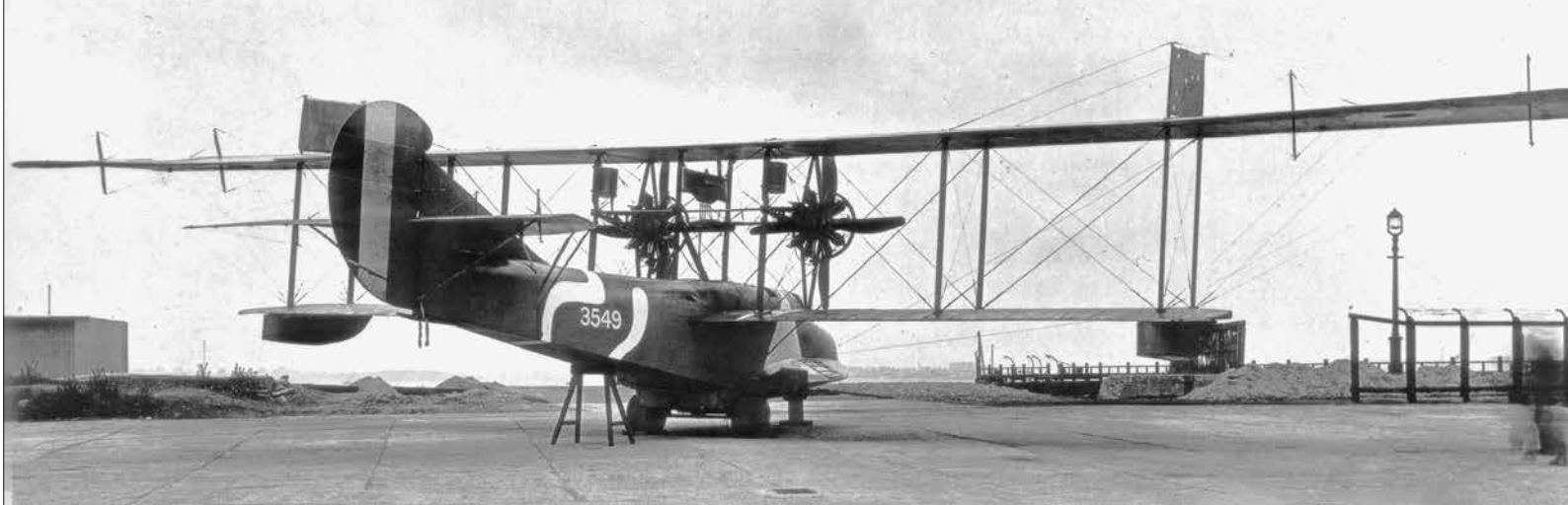
Curtiss H.4 3549 on the ramp at Felixstowe, clearly showing the twin Anzani radial engines.
