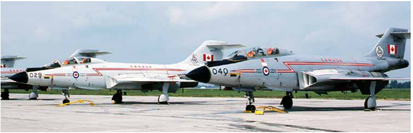
Two 416 Squadron Voodoos at CFB Trenton, September 1980, in contrasting overall colour schemes. 101040 is shown in the aluminum lacquer overall colour scheme, and 101029 with the Alumigrip light grey enamel as applied after 1980. Also note the IR sensor head mounted externally on the nose just forward of the canopy. BILL CUMMING
