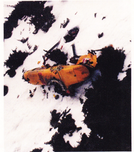
The crumpled and burnt wreck of Rescue 311 lays where it stopped following its 500-foot roll down a mountainside. The photo does not reveal the steepness of the slope which necessitated the use of ropes to move about during the recovery operation (Photo courtesy of Air Detachment, RCMP)
