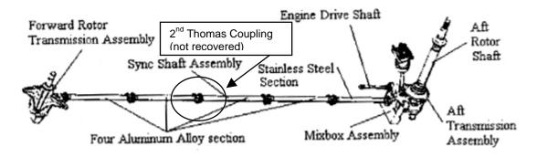
Figure 2: Sync Shaft and Transmission Assemblies
