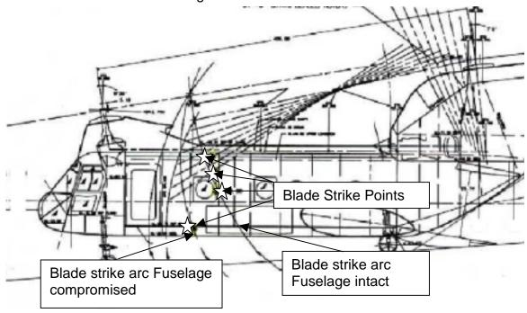
Figure 4: Pylon position and blade arcs compared to fuselage strike positions
