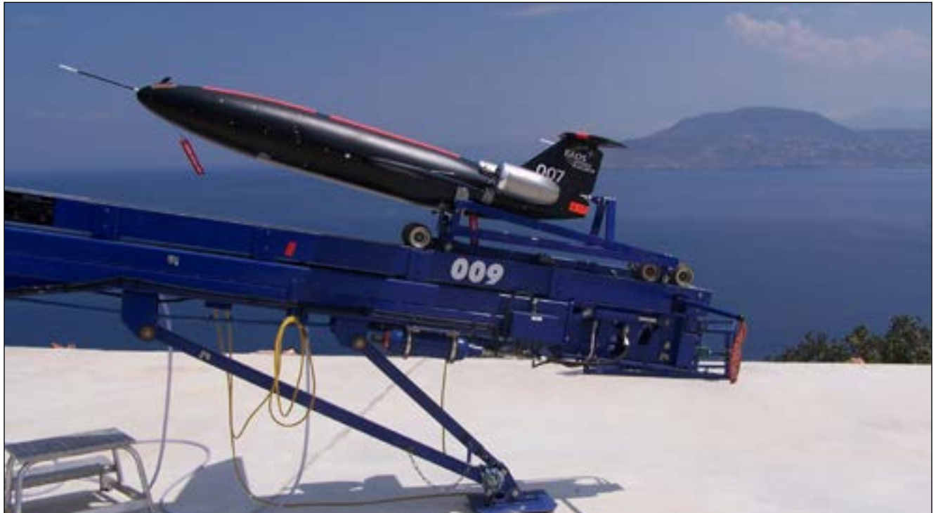
A view of the DO-DT45 drone similar to the Meggit Training Systems Hornet target drone employed in Canadian service. Recovery of the drones is achieved with parachutes. (CF Photo courtesy of EADS)
