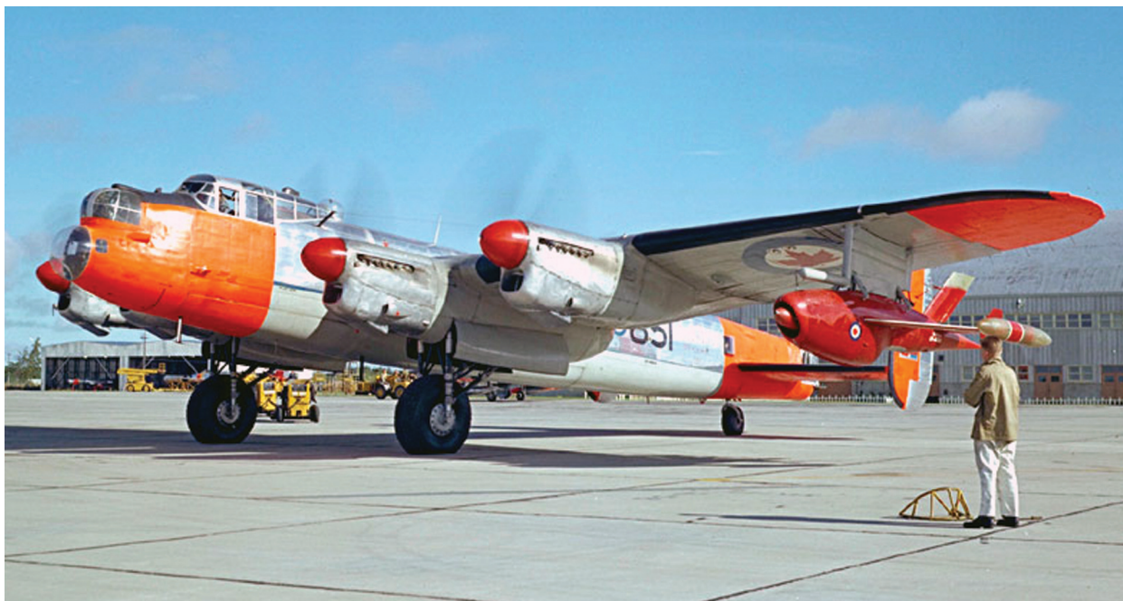
Two RCAF Lancaster Mk10s were modified as launch and control platforms for Teledyne-Ryan Firebee drones in Canadian service. Recovery of the drones was achieved with parachutes. (CF Photos)
