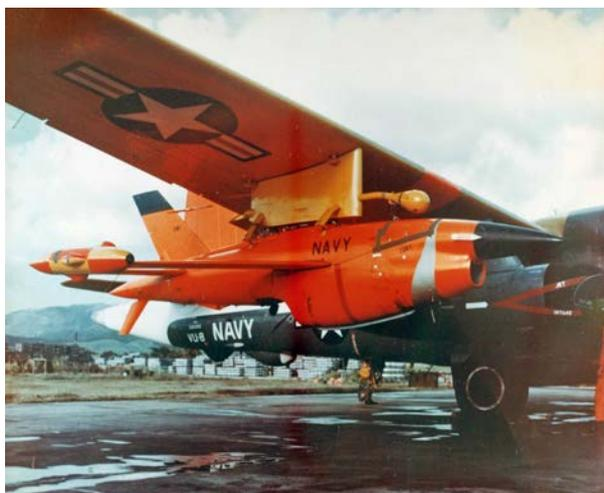
*The later generation BQM-34 Firebee is shown here mounted under the wing of a USN Neptune. - (USN Photo)*
