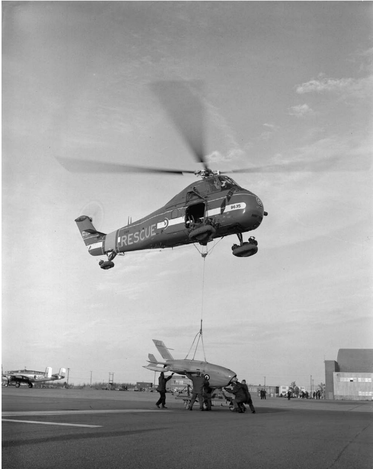
*The KDA-4 Firebee is shown here being manhandled onto its ground handling cradle - (RCAF Photo - PL-120089)*
