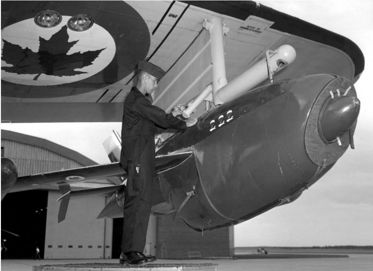
**A fine close-up of the RCAF KDA-4 Firebee mounted on the wing launch rack underneath a Lancaster. Note the white mission markings on the centre fuselage. A protective cover has been installed over the jet engine inlet. - (RCAF Photo)**
