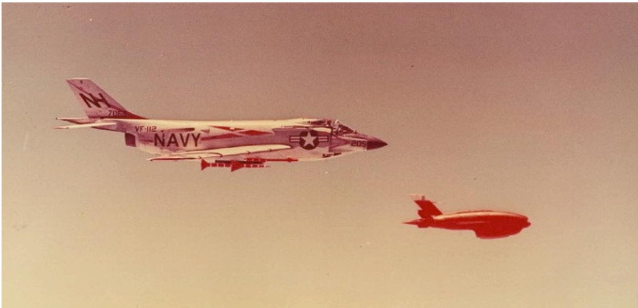
*A fine close-up of a KDA-4 Firebee flying alongside a US Navy Demon jet fighter carrying both a Sparrow and Sidewinder missile. In 1960, the RCAF cooperated with the US Navy providing Firebees for test firings of the Sparrow III missile from Demon aircraft at Cold Lake in a test program known as Operation "Blue Tar". - (USN Photo)*
