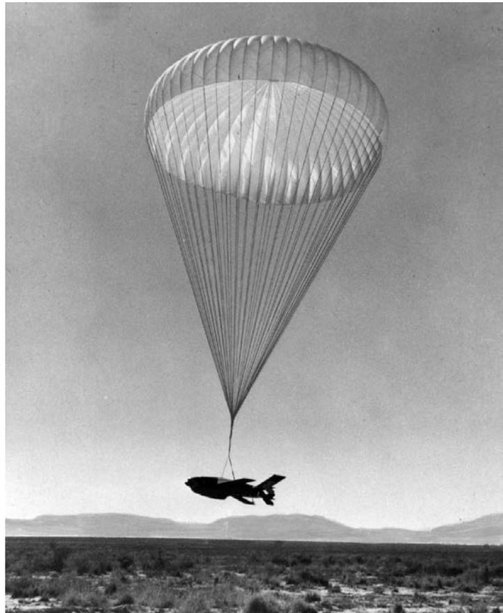
*The Firebee design employed a two-stage parachute system; a drogue chute to slow the drone and a much larger canopy, as seen here, to safely lower it to the ground - (Photo courtesy of the San Diego Air and Space Museum Archives)*
