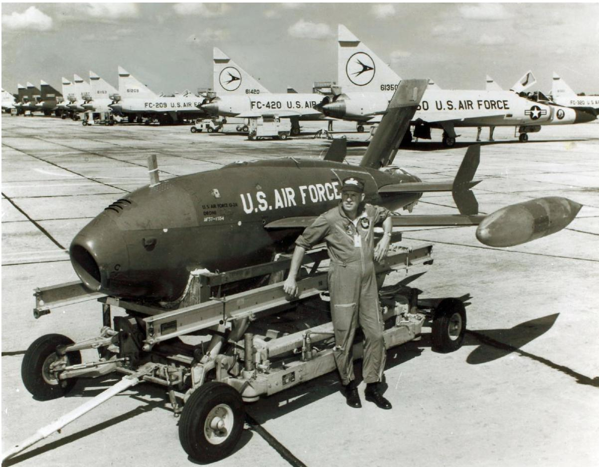
*The USAF's Q-2A Firebee drone is illustrated in the above photo. Note the absence of a nose inlet centre body and the radar reflector pod on the wing tip. The Q-2 A, B and C variants were all powered by Continental J-69 jet engines. - (USAF Photo)*
