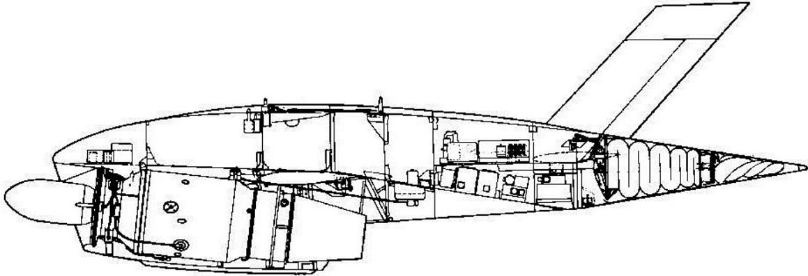
*A cross-sectional view of the KDA-4 clearly illustrates the engine installation (note the inlet centre body) along with the avionics bay and parachute installations towards the rear of the fuselage. - (Ryan Aeronautical Company drawing courtesy of the San Diego Air and Space Museum Archives)*
