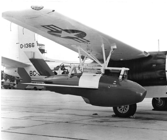
**The Firebee is shown here mounted under the wing of a USAF A-26 Invader. - (USAF Photo)**
