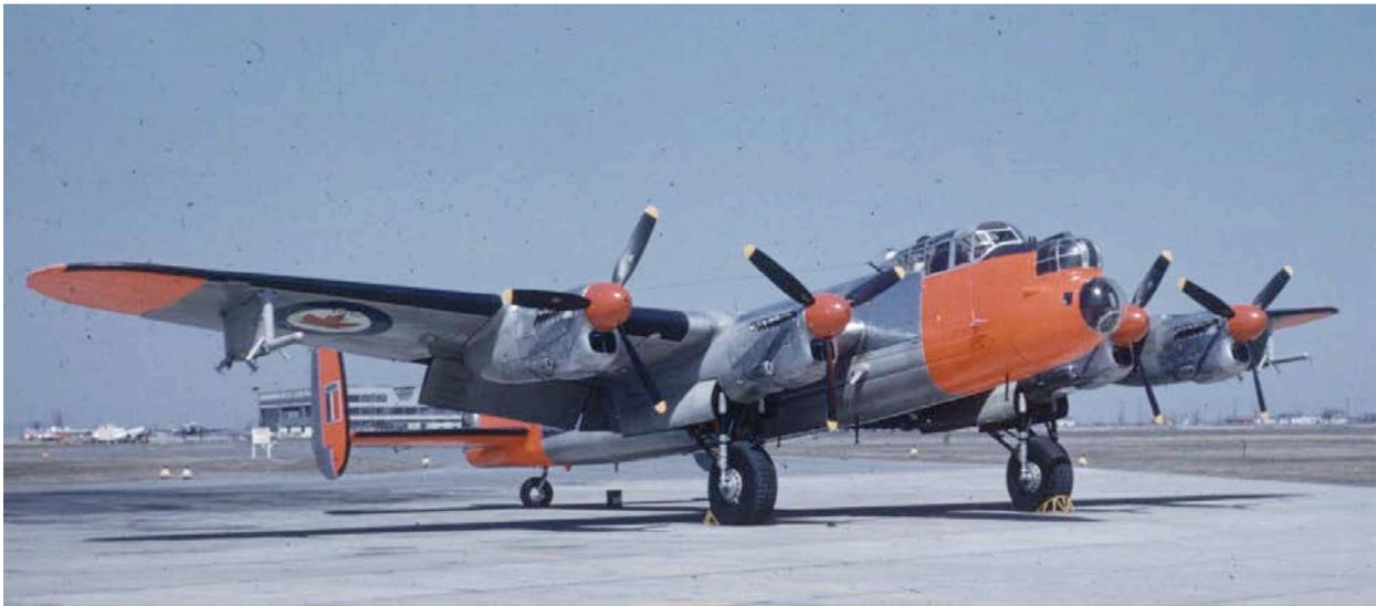
*One of two RCAF Lancaster drone controller aircraft shortly after conversion. Note the drone pylon / carriage racks under each wing and the non-standard, high-visibility paint scheme. - (RCAF Photo)*
