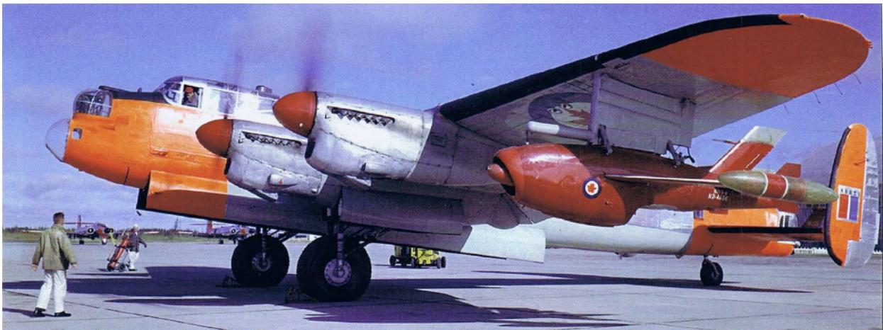
*Another fine view of the RCAF KDA-4 Firebee mounted on the wing launch rack underneath Lancaster KB851 . Note the wing-tip mounted electronic reflectors on this particular Firebee. - (RCAF Photo)*
