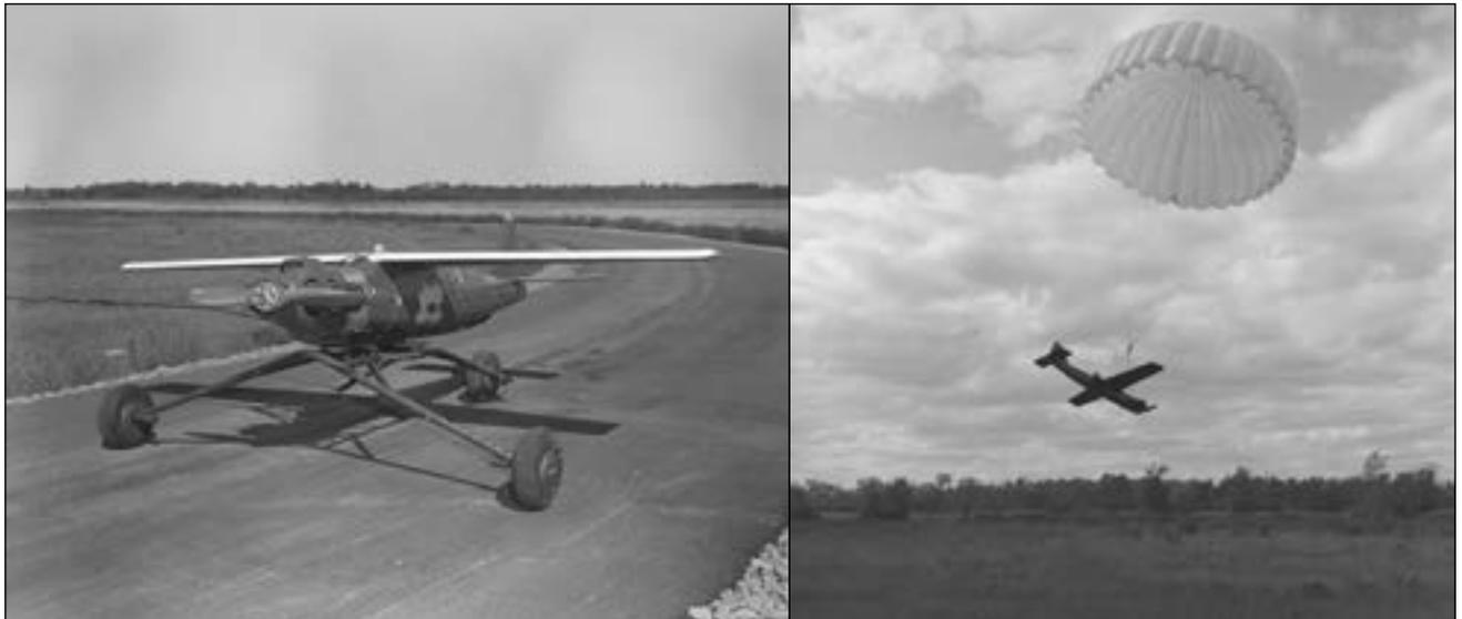
*Two views of the little known Radioplane OQ-19 target drone being tested by the RCAF in these photos - (CF Photos)*
